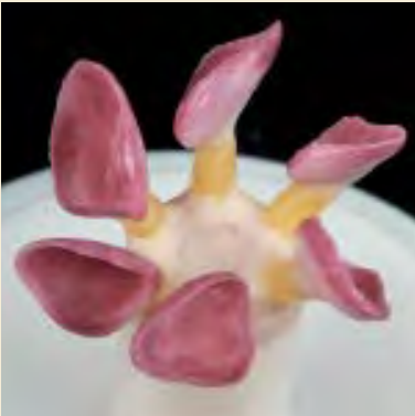
Fig 5a Waxed dies in position to be placed in the investment cylinder.
